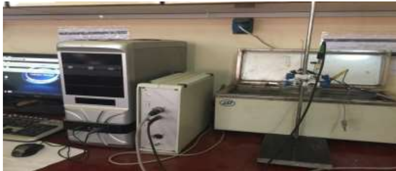
Figure (6): Corrosion rate device type (X MTD-2MA).
